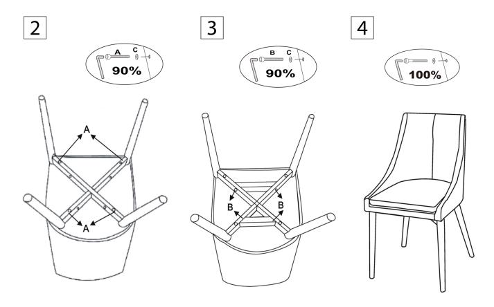
Finally, level the chair and tighten all the bolts 100%
